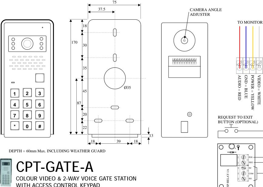
A 12 volt power supply must be connected to the +12VDC INPUT (COM) for the Keypad to work. This can either be taken from the monitors power supply, down an extra wire, or from the power supply that runs door the lock.
